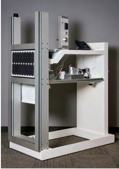
A mock-up demonstrating connected devices including: security, telecom, lighting, cooling, a motorized roller shade and solar panels that follow the sun and feed power back to the ISP panel.
